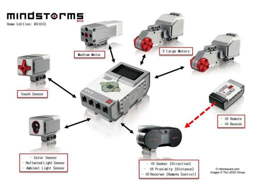
Fig 1: Main components of EV3 robot
